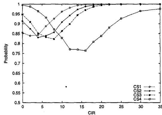
Figure 11 Probability  $P_c$  for 50 km/h, a spacing of 4 slots and different CSs
