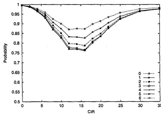
Figure 10 Probability  $P_c$  for 50 km/h and CS4
