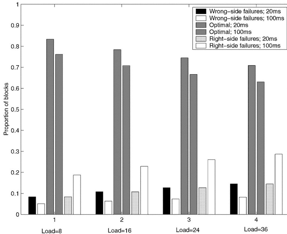
Figure 2. Optimal, right and wrong side failures for updating periods of 20 and 100 ms and various loads.
