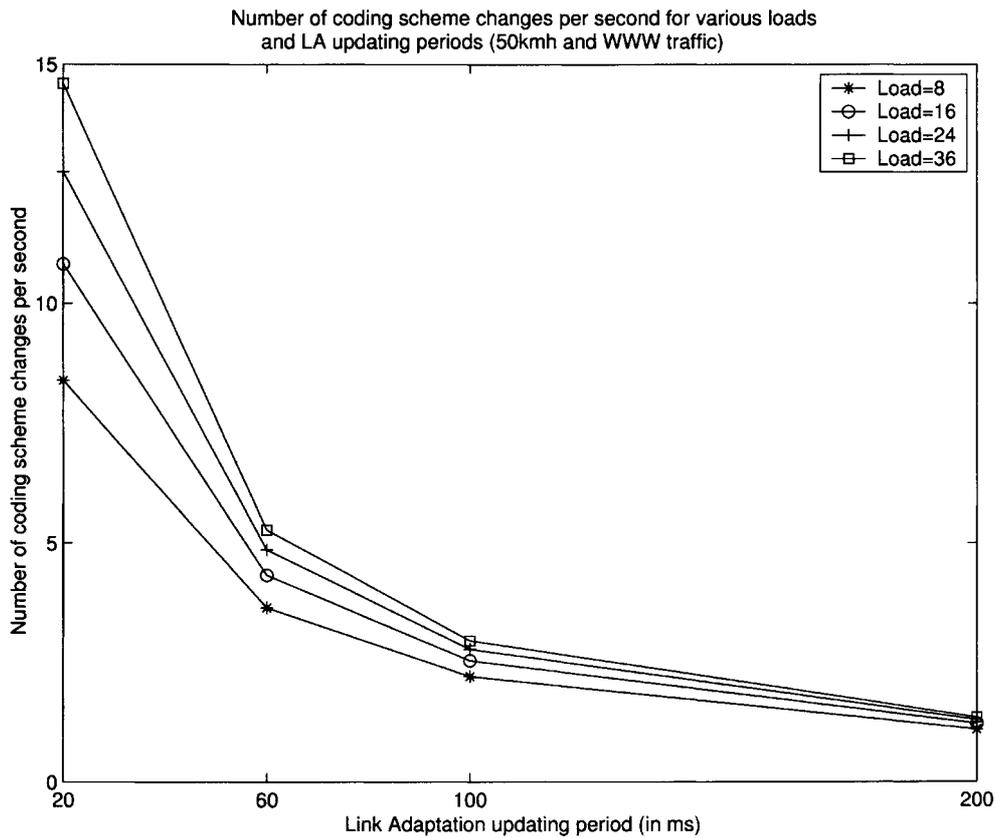
Figure 3. Number of CS changes (WWW traffic, 50 km/h).
