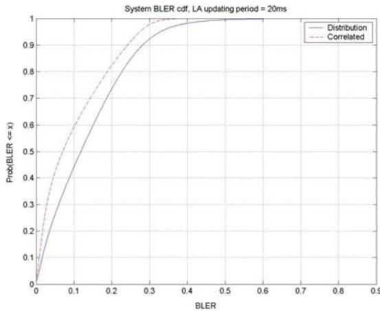
Figure 8 – System BLER cumulative density function for a LA updating period of 1 RLC block (20 ms).
