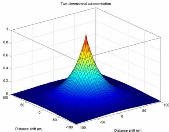
Figure 2: Autocorrelation of shadowing as a function of distance shift (movement in two dimensions).
