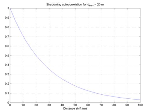
Figure 1: Shadowing autocorrelation function
