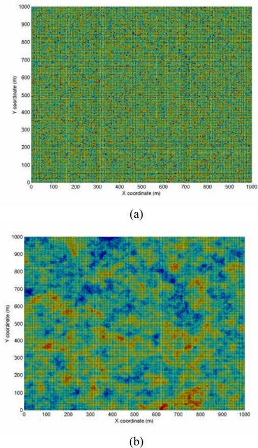
Figure 3: (a) Unfiltered and (b) filtered 2D shadowing maps.
