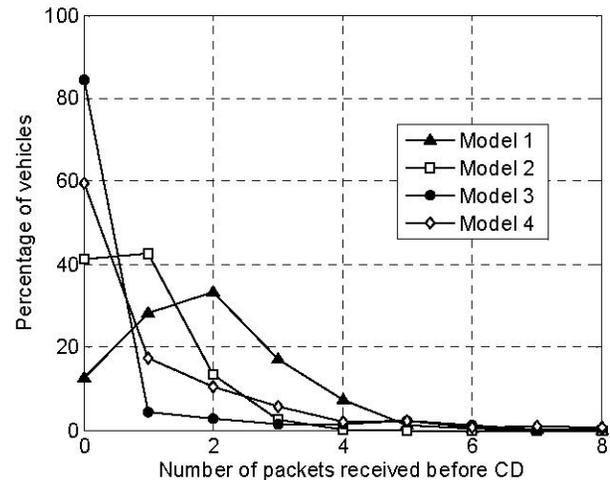
Fig. 5. Percentage of vehicles that receive a particular number of messages before the critical time corresponding to a  $RT=1.5s$  ( $P_t=0.75W$ ).
