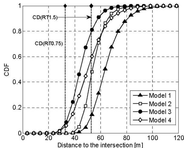
Fig. 4. CDF of the distance at which the first message is received ( $P_t=0.75W$ ).
