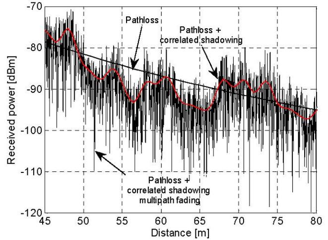
Fig. 1. Wireless propagation effects on the received power [dBm].
