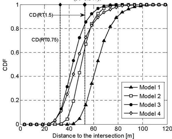
Fig. 8. CDF of the distance at which the first message is received under high channel load ( $P_t=0.75W$ ).
