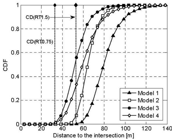
Fig. 7. CDF of the distance at which the first message is received ( $P_t=1.5W$ ).
