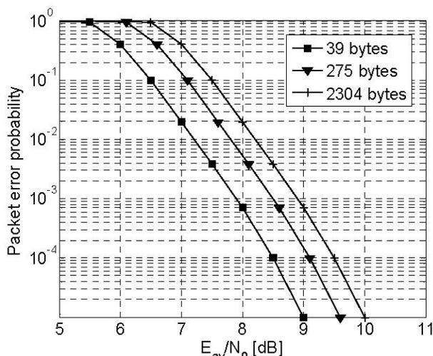
Fig. 3. Packet Error Rate for the WAVE 6Mbps transmission mode (QPSK and  $\frac{1}{2}$  coding rate)
