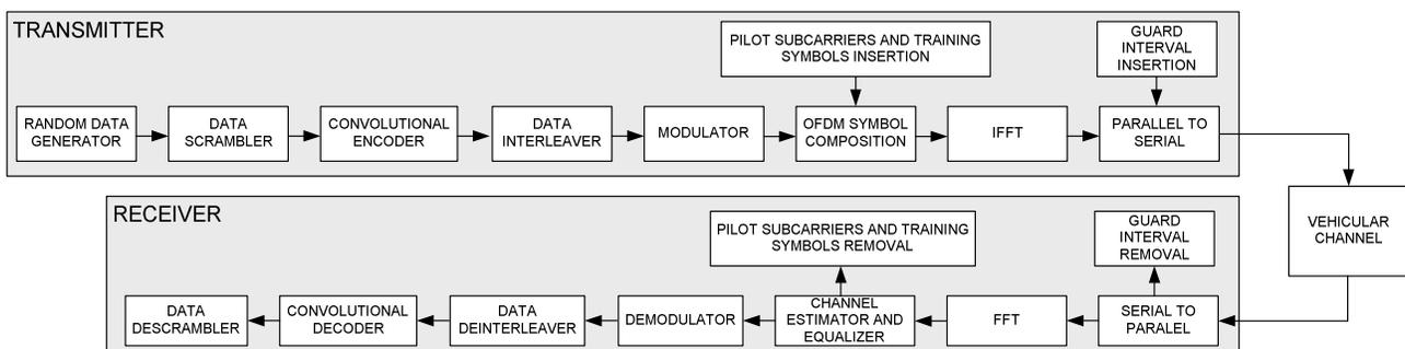
Figure 2. ITS-G5A PHY layer block diagram.
