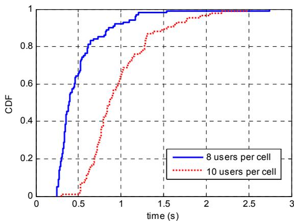
Figure 6 – CDF of the CCNT-derived real computational time (s) for the JRRM Max\_MinU proposal considering the TMS320C6455.
