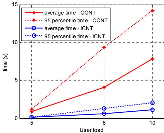
Figure 3 – Time needed by the Max\_MinU algorithm to find a JRRM optimal solution using the DSP56311.
