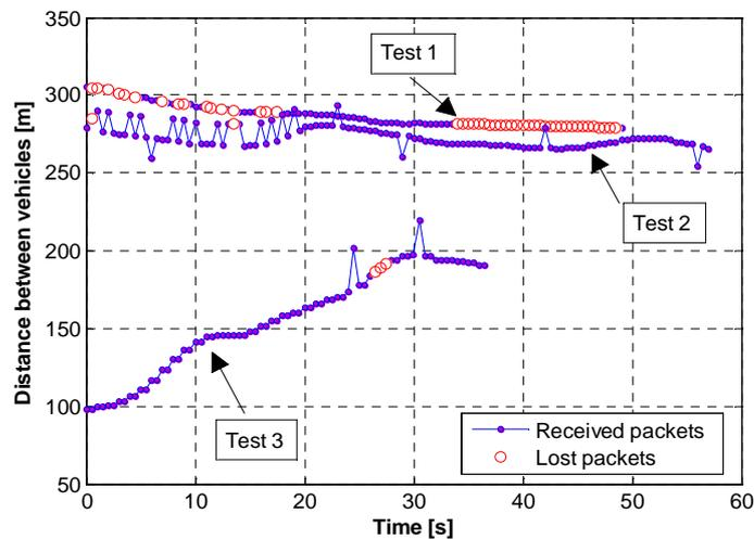
Figure 5. Distance between the two vehicles for the car-following communications assessment tests
