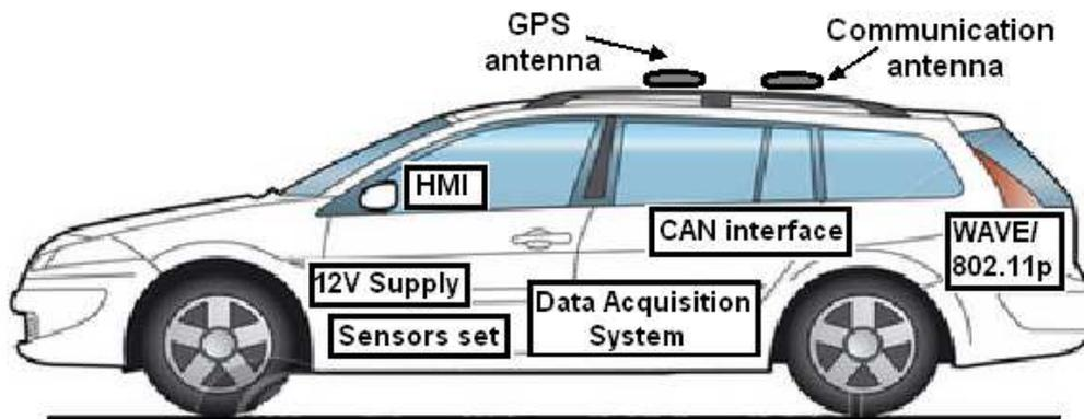
Figure 4. Schematic of a vehicle instrumented with an OBU Cooperative ITS prototype
