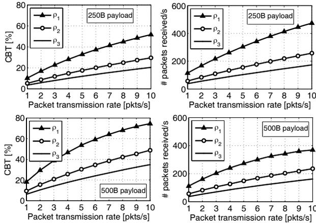
Fig. 3. Channel busy time (CBT) and number of packets correctly received per second for the CAM configurations that satisfy the application requirements with the target reliability ( $D_w$ ,  $p_{app} = 0.99$ ), considering  $TWindow = 2s$  and varying vehicular density  $\rho$ .
