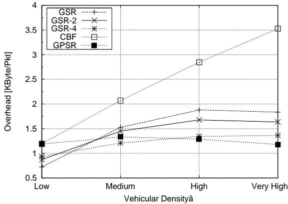
Fig. 4: Protocol overhead under uniform traffic conditions (*Manhattan-A*)
