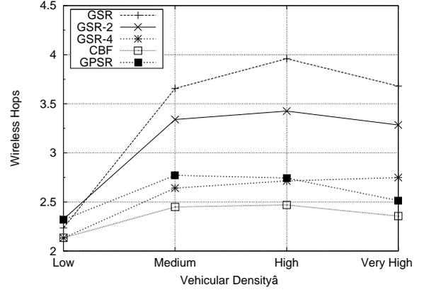
Fig. 5: Wireless hops under uniform traffic conditions (*Manhattan-A*)
