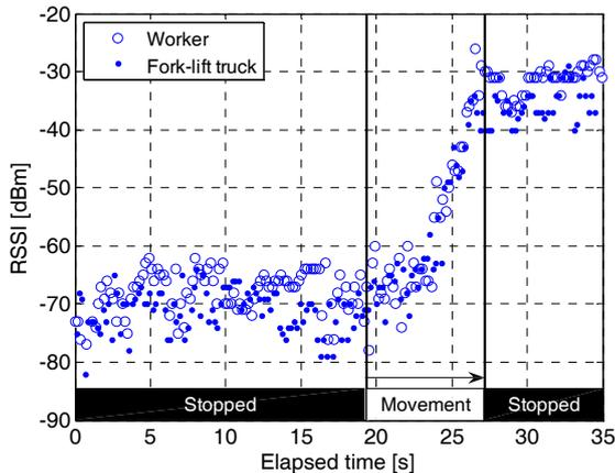
Figure 7. RSSI of the received packets for the collision avoidance use case.  $P_t=3\text{dBm}$ ,  $h_w=1.2\text{m}$ ,  $h_f=1.8\text{m}$ ,  $T=200\text{ms}$ ,  $\text{payload}=50\text{Bytes}$ .
