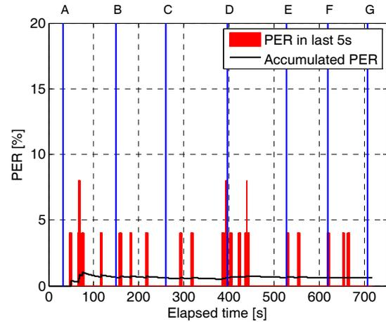
Figure 5. Packet Error Rate experienced as the mobile transmitter node moves across GORATU's factory.  $P_t=3\text{dBm}$ ,  $h_t=1.2\text{m}$ ,  $h_R=5\text{m}$ ,  $T=200\text{ms}$ ,  $\text{payload}=50\text{Bytes}$
