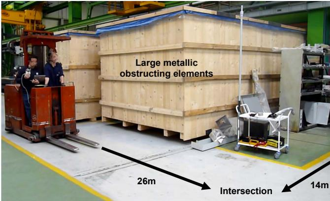
Figure 6. Image of GORATU's factory with the trajectories of the two nodes emulating the collision avoidance use case.
