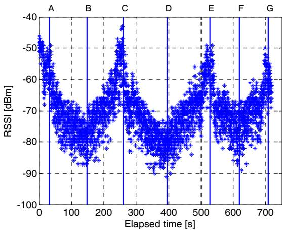
Figure 4. RSSI of the received packets as the mobile transmitter node moves across GORATU's factory.  $P_t=3\text{dBm}$ ,  $h_t=1.2\text{m}$ ,  $h_R=5\text{m}$ ,  $T=200\text{ms}$ ,  $\text{payload}=50\text{Bytes}$ .
