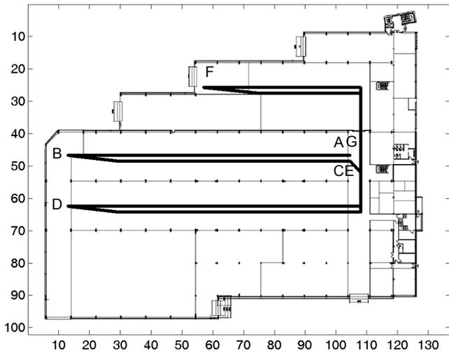
Figure 3. Movement of the transmitter node across GORATU's factory.
