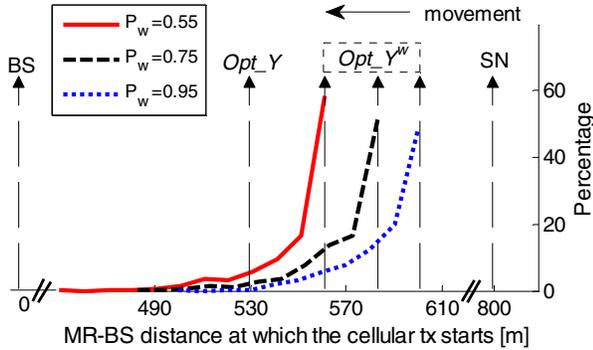
Figure 2. Distribution of the locations at which MR initiates the cellular transmission to the BS ( $\lambda=1/3s^{-1}$ ) for the ‘Opt-PRBs’ scheme.
