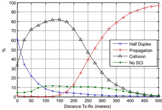
Fig. 8. Percentage of TBs incorrectly received per type of transmission error as a function of the distance between transmitter and receiver (values estimated with respect to  $N_{error}$ ). Single SCI+TB transmission per packet.
