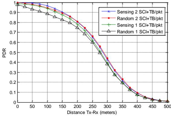
Fig. 4. PDR as a function of the distance between transmitter and receiver under LOS conditions.
