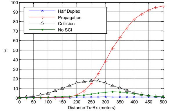
Fig. 7. Percentage of TBs incorrectly received per type of transmission error as a function of the distance between transmitter and receiver (values estimated with respect to  $N_{total}$ ). Single SCI+TB transmission per packet.
