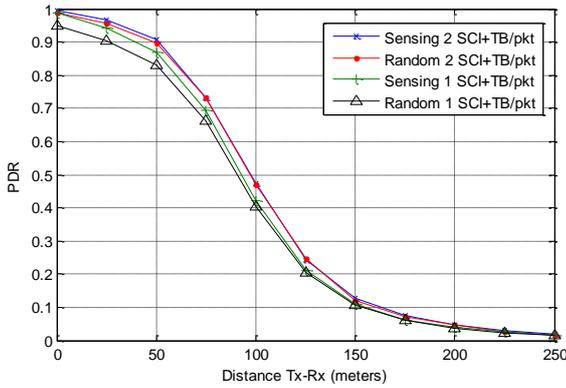
Fig. 5. PDR as a function of the distance between transmitter and receiver under NLOS conditions.
