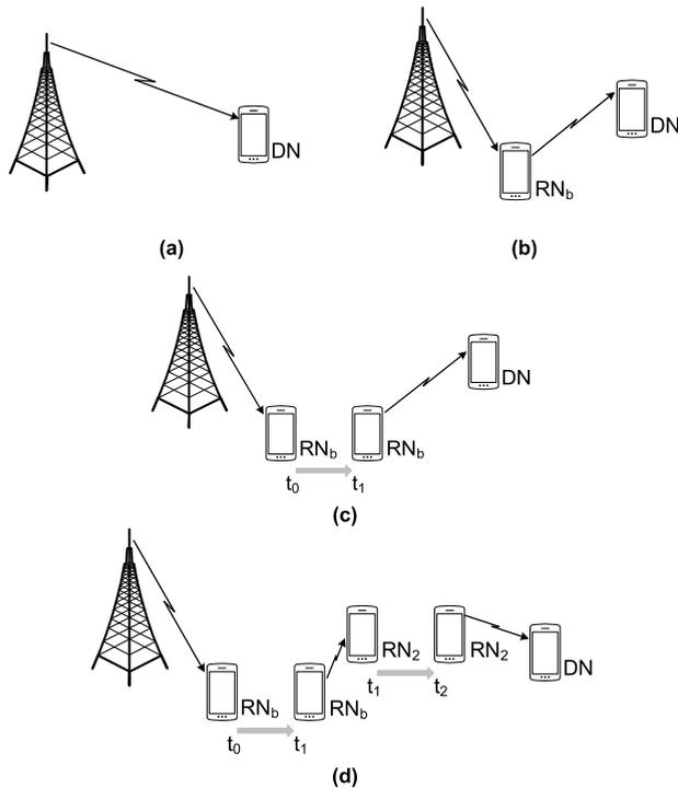
**FIGURE 1. Illustration of communication modes. (a) SH communication; (b) MH communication; (c) 2-hop MH-OPP communication; (d) 3-hop MH-OPP communication.**
