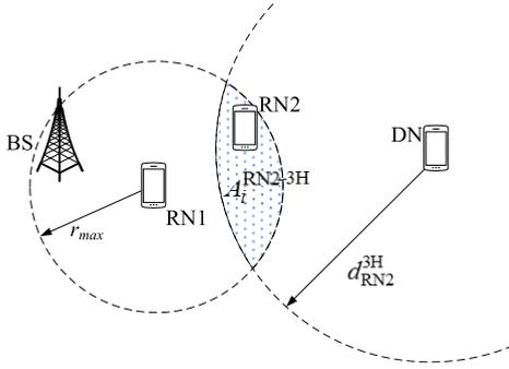
**FIGURE 4.** Illustration of  $A_i^{RN2-3H}$  for condition #3 that RNs must satisfy to establish an 3-MH-OPP connection.
