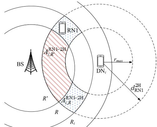
FIGURE 3. Illustration of  $A_i^{RN1-2H}$  RN1-2H for condition #2 that RNs must satisfy to establish an 2-MH-OPP connection.
