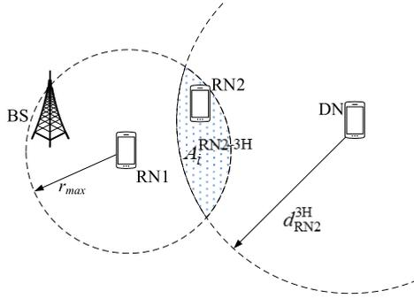
**FIGURE 4.** Illustration of  $A_i^{RN2-3H}$  for condition #3 that RNs must satisfy to establish an 3-MH-OPP connection.
