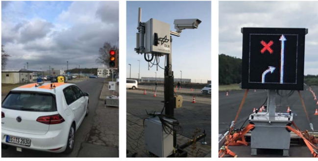
Fig. 2. DLR's FASCarE in front of the mobile traffic light (left), the mobile RSU (middle) and the used VMS (right).
